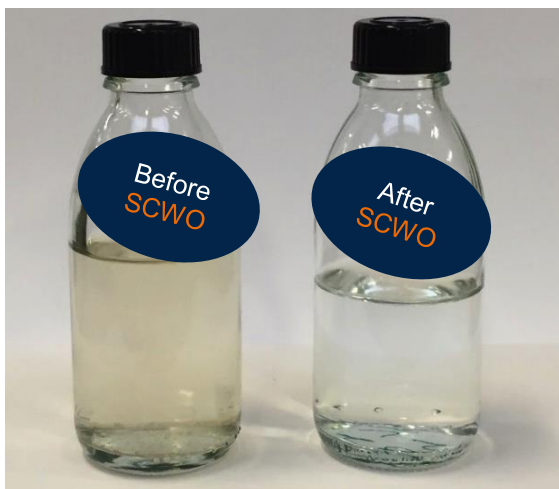
It is clear to see the difference between the wastewater before and after SCWO treatment.
