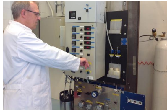
Aquarden's Chemical Technician in front of the laboratory reactor, where the tests of SCWO treatment of hospital wastewater, with more than 60 drug residues, took place. The unit is a small replica of the full-scale SCWO system plant.
