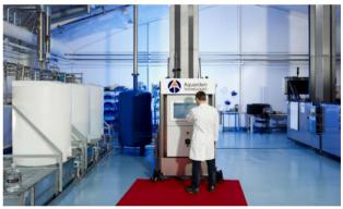
The modular on- or offsite SCWO-system, SuperOx<sup>®</sup> completely destroys hardly-degradable and hazardous pollutants in industrial wastewater.
