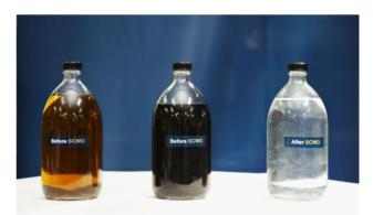
Leachate from landfill before and after treatment in Aquarden's SCWO system, SuperOx<sup>®</sup>. The result is pure water that can be discharged to receiving water bodies.
