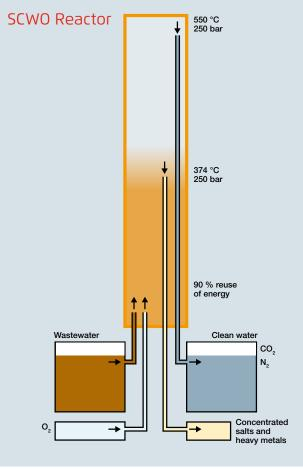
The SCWO reactor principle: Salts and heavy metals are concentrated and removed at a temperature of around 374 °C while organics oxidize further up in the reactor at 450-550 °C.
