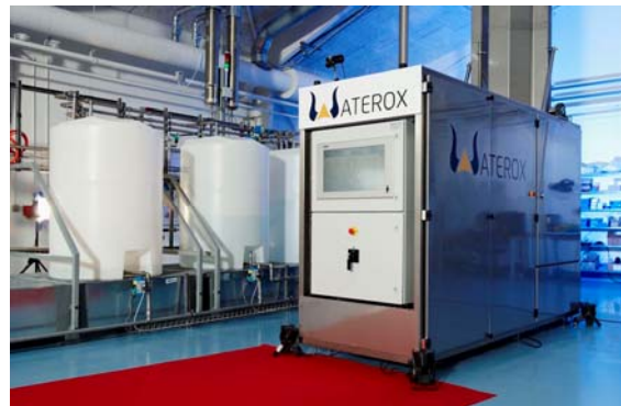
Aquarden's SCWO-based Waterox system is designed to treat the most problematic wastewater streams from e.g. pharmaceutical, biotech, and chemical industries. The system received 'The European Business Award for the Environment 2016' in Denmark and is given to a new and innovative product that significantly contributes to sustainable development and innovation.
