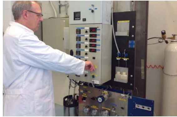
Aquarden's Chemical Technician in front of the laboratory reactor, where the tests of SCWO treatment of hospital wastewater, with more than 60 drug residues, took place. The unit is a small replica of the full-scale Waterox plant.
