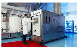
The modular and onsite Waterox-system completely destroys hardly-degradable and hazardous pollutants in industrial wastewater.
