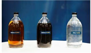
Leachate from landfill before and after treatment in Aquarden's Waterox system. The end product is pure water that can be discharged to receiving water bodies.
